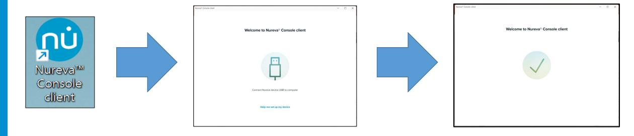
Install Nureva Console client then launch the Console client app. Connect the Nureva connect module to the PC with a USB cable.
